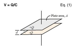
A simple form of a capacitor consists of two parallel conducting plates, each with area A, separated by a distance *d*. The charge is uniformly distributed on the surface of the plates. The capacitance of this parallel-plate capacitor is given by:
