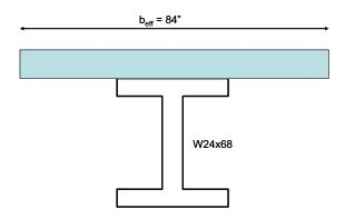
2. Determine if the composite beam pictured below is adequate for this application (this includes bending, shear, deflection and shear stud limit states). The dead load for this beam is 10 psf plus the weight of the deck, which is made from normal weight concrete.
