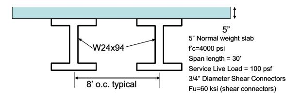
3. <u>Given:</u> The sketch and details below (which is identical to the information provided in Problem #1). The span of the beam is 35 feet, the beams are spaced 7 feet apart and the beam supports a live load of 100 psf in addition to the dead load of the slab which is comprised of light weight (density = 125 pcf) concrete. <u>Find:</u> The number of required shear connectors for fully composite action of a typical interior beam. Your stud design should comply with AISC I8-1. In addition to
